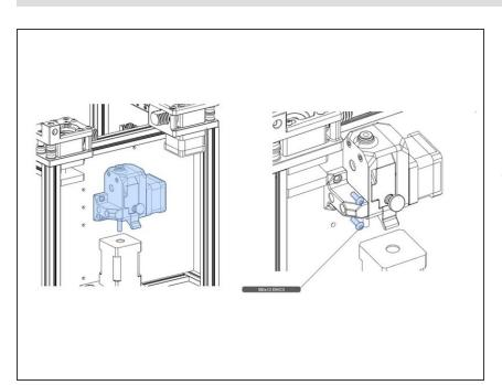
Attach the extruder through the back panel into the Z vertical extrusion.
