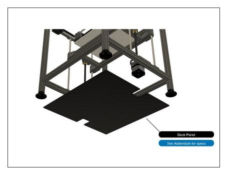
If you use the RepRap display from the previous step, you will need to remove it to slide the deck panel in place.
