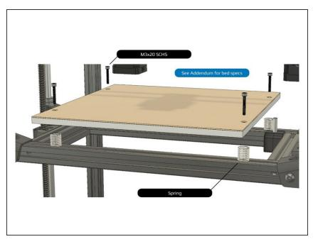
• Bed power wires should be oriented towards the rear of the printer.
