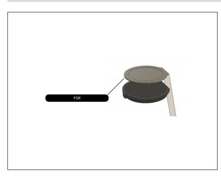
• Most FSR pads have a sticky backing. Peel carefully.
