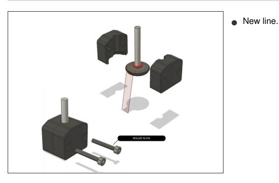
Step 4 — Attach FSR to Bed Carrier
