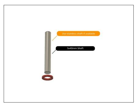
Printed pin retainer should fit snugly to prevent pin from falling out when machine is flipped.
