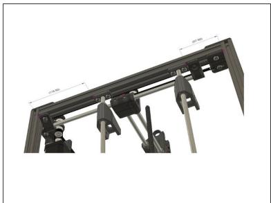
Use calipers to measure 8mm rod placement.
