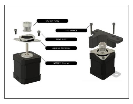
If you opt out of using dampeners, you may need to adjust or rotate the 20t pulley.
