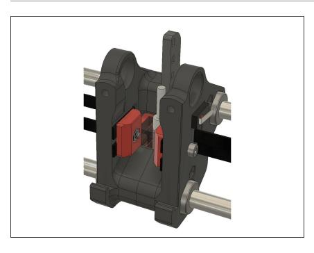
Start at the carriage. Set the belt flush to the edge and tighten the belt retainer. **07 - Run the Belts**Guide ID: 38 - Draft: 2020-02-08
