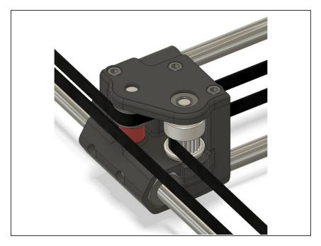
Run the belts to the X/Y joints. The toothed side should run against the 20t pulleys. The smooth side should run against the flanged bearings.
