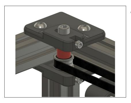
Run one belt to the front idler/tensioner and back to the X/Y joint. **07 - Run the Belts** Guide ID: 38 - Draft: 2020-02-08
