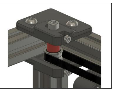
• Run the belts down the other side through the X/Y joint and front idler.
