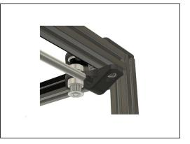
Ensure smooth movement on both axis before tightening down to the frame.
