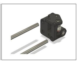
Be sure to lube the bearings before adding the 8mm rods.
