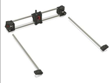
Be sure to add lube to the bearings before assembly.
