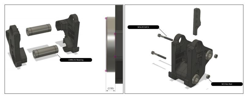
• Be careful not to crack the carriage pieces when inserting the bearings.
