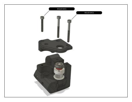
Be careful not to over-tighten screws into plastic.
