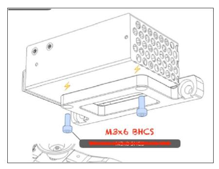
Use M3x6 BHCS when mounting RS-25-5 PSU. M3x8 may go too far into the PSU body and puncture the insulating sheet, shorting out the main PCB.
